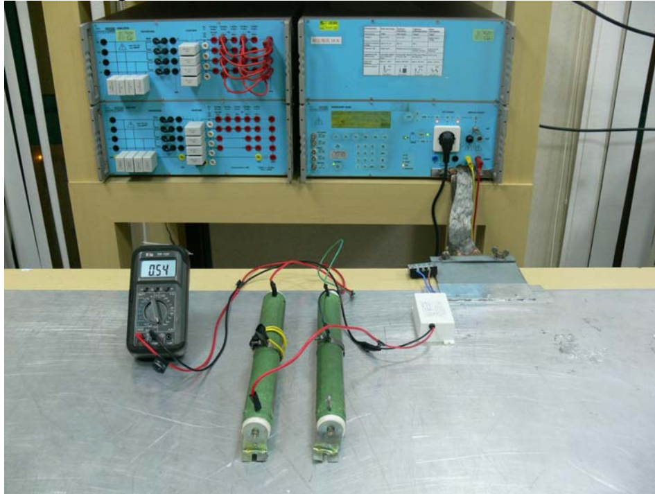
Set Up Photo of Surge & V-DIPS
